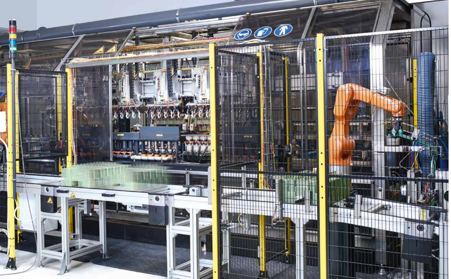
Plant for plating single valves for the automobile industry in Holzapfel Group's Fast Plating Center
